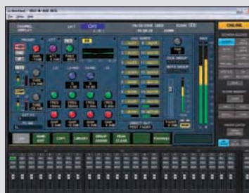
M-400RCS remote control software. You can setup configurations and channels ahead of time, save existing projects and adjust any type of mixer setting, recall scenes, load presets, etc.
