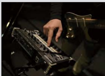
The M-48 can be attached to a mic stand using a mounting bracket. LED equipped encoders are ideal for easy operation in darkened venues.
