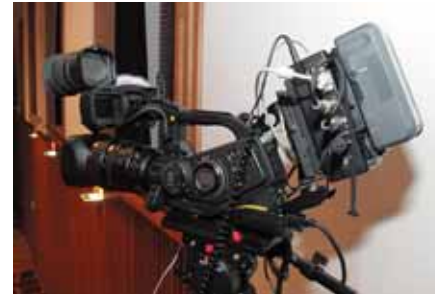
Using the F1-VMK1 V-mount accessory, the F-1 and V-mount battery can be mounted on the back of a camera.
