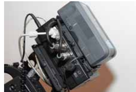
Line audio from the mixing console was fed to the F-1 mounted on the rear of the XL H1S.
