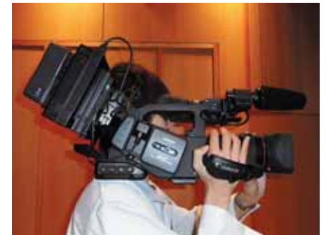
Example of shooting with a shoulder-mounted camcorder in combination with an F-1 and V-mount battery.
