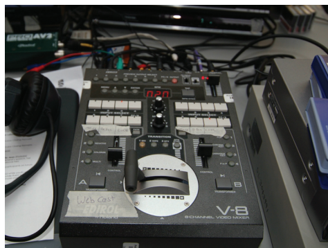
The V-8 was used for live switching and webcast mixing.
